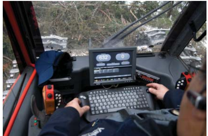
Figure 1. In a Valmet 941.1 wood-logging harvester, the operator looks at two things: the forest and his computer screen. On the computer screen is displayed all sorts of information concerning, amongst others, the trees (length, specie, assortment, etc.), price lists, maps, and machine settings.
