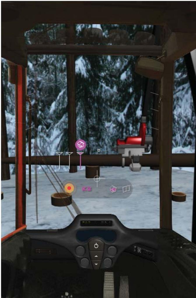
Figure 3. Visualization of the main information on the head-up display.
