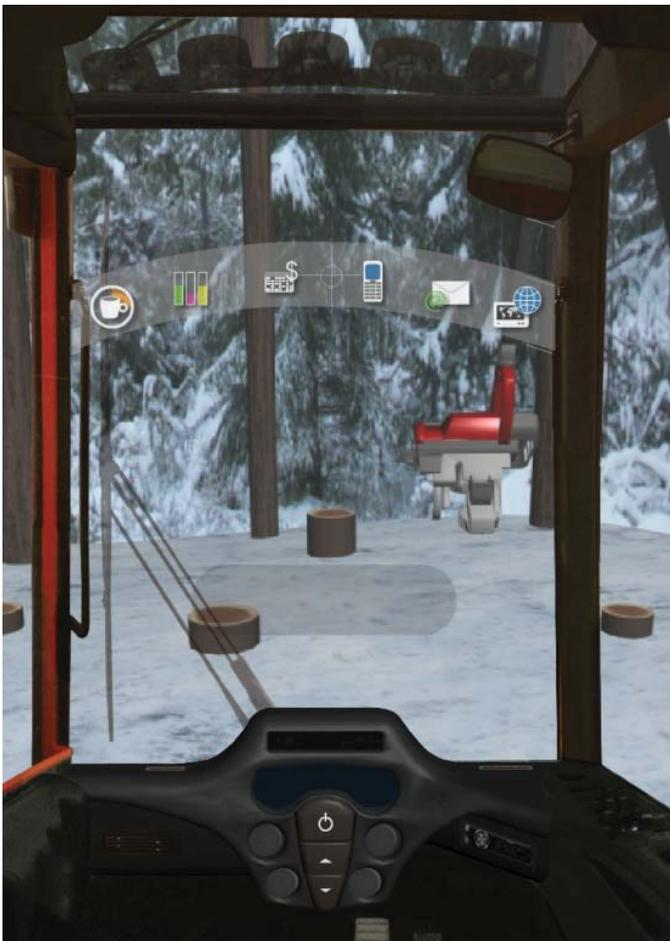
Figure 5. Visualization of the machine information (group 3) on the head-up display.
